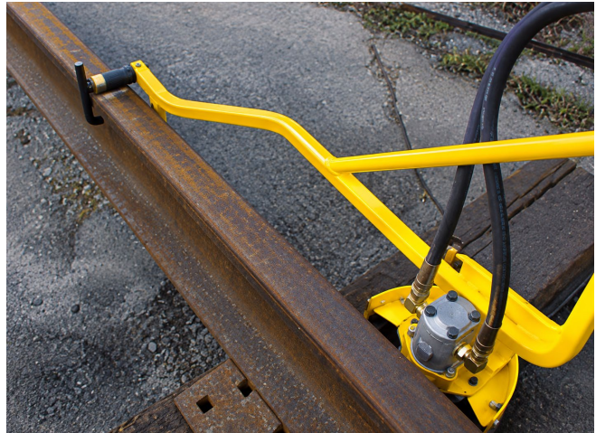
Web Grinder on the rail.
