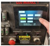
9. Enter the pin code **2156** to Unlock Calibration.
